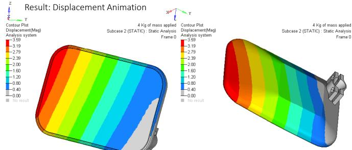
Due to application of 4 Kg mass, maximum displacement observed in mirror is about 3.59 mm at free edge and zero at fixed end
